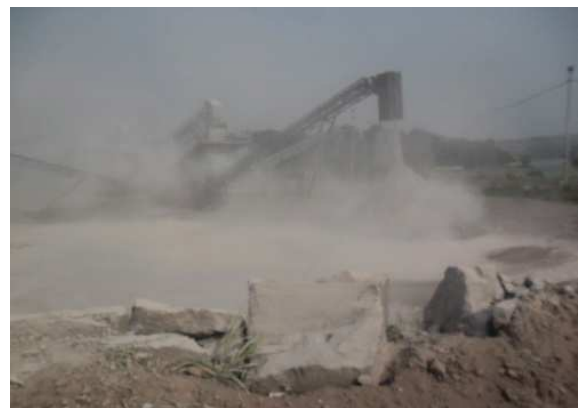
Figure 21. Dust emission from crushing of aggregates (Kombé).
