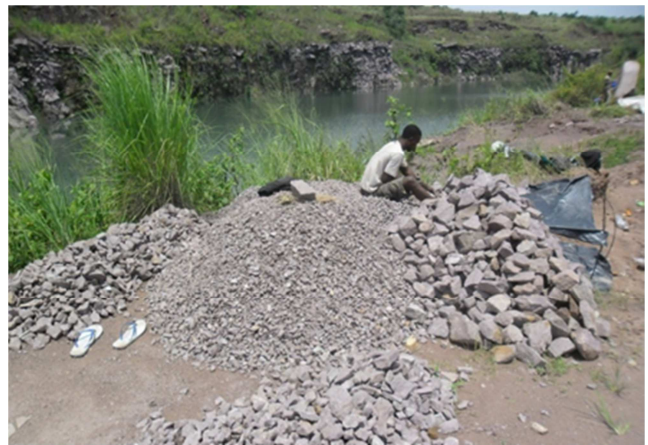
Figure 10. Artisanal processing scene: manual crushing of aggregates (Kombé, Brazzaville).
