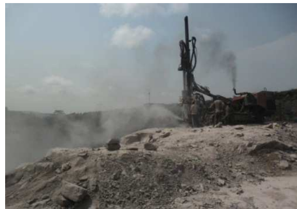
Figure 20. Dust emission from drilling of mine holes (Kombé).
