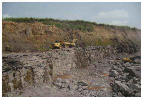
Figure 26. Stripping of the sterile level (Kombé).
